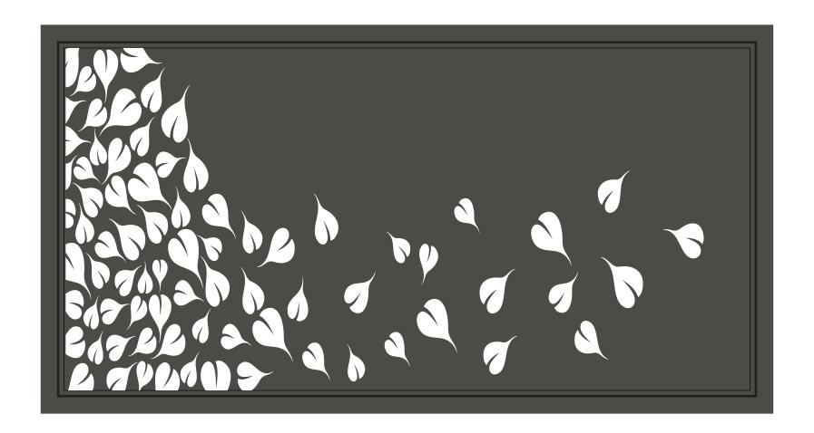
MAIN FRAME - Easy gate main frame 92x48x3. Mitred corners with welded 3mm thick corner braces giving 6mm wall thickness at each corner. INFILL - Water jet panel design 0022 in 3mm aluminium. Back brace over 3150mm wide. Easy rubber finishing insert. FINISH - Pre treatment and powder coat. Kit includes covers to conceal all infill fastening points. SIZE RESTRICTIONS - Sliding maximum width 6450mm. Swing maximum width 3200mm. Maximum height 1650mm.
