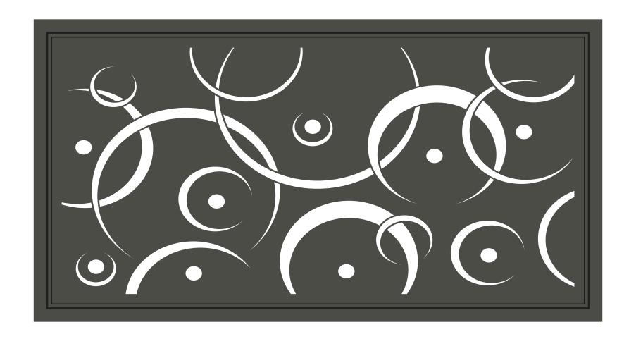
MAIN FRAME - Easy gate main frame 92x48x3. Mitred corners with welded 3mm thick corner braces giving 6mm wall thickness at each corner. INFILL - Water jet panel design 0018 in 3mm aluminium. Back brace over 3150mm wide. Easy rubber finishing insert. FINISH - Pre treatment and powder coat. Kit includes covers to conceal all infill fastening points. SIZE RESTRICTIONS - Sliding maximum width 6450mm. Swing maximum width 3200mm. Maximum height 1650mm.
