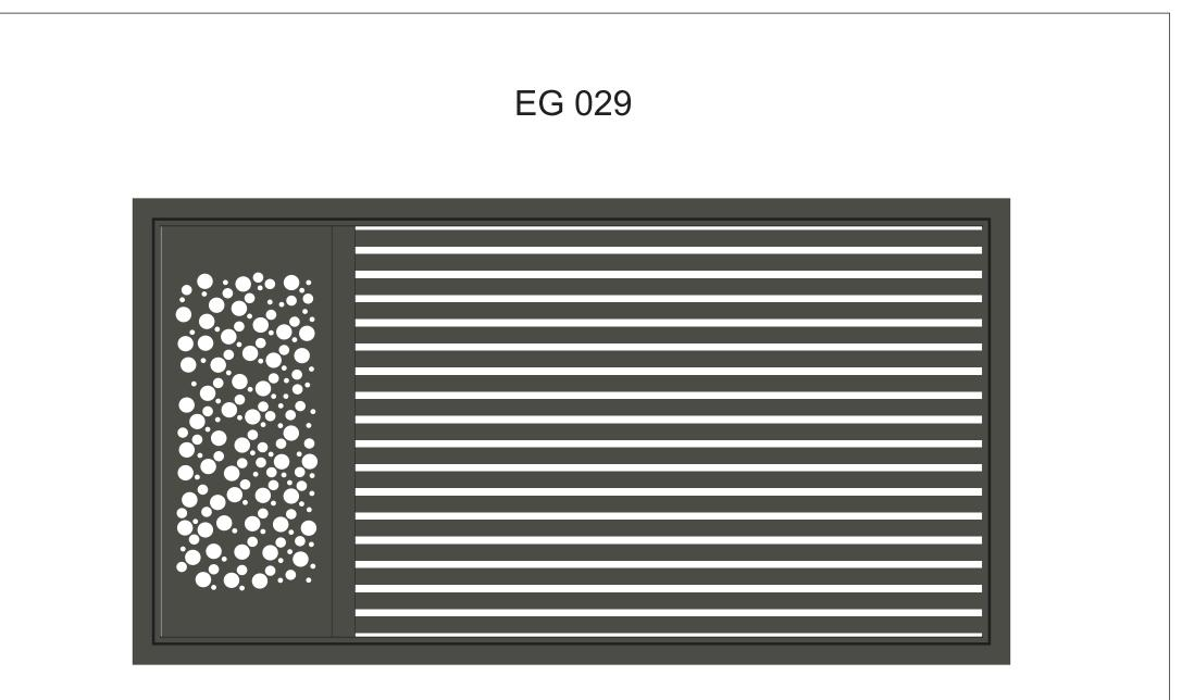
MAIN FRAME - Easy gate main frame 92x48x3. Mitred corners with welded 3mm thick corner braces giving 6mm wall thickness at each corner. INFILL - 65x16 horizontal slats at nominal 15mm spacing (adjust to suit your requirements). Decorative panel can be adjusted to anywhere in the gate. FINISH - Pre treatment and powder coat. Kit includes covers to conceal all infill fastening points. SIZE RESTRICTIONS - Sliding maximum width 6450mm. Swing maximum width 3200mm.
