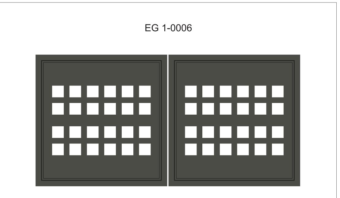
MAIN FRAME - Easy gate main frame 92x48x3. Mitred corners with welded 3mm thick corner braces giving 6mm wall thickness at each corner. INFILL - Water jet panel design 0006 in 3mm aluminium. Back brace over 3150mm wide. Easy rubber finishing insert. FINISH - Pre treatment and powder coat. Kit includes covers to conceal all infill fastening points. SIZE RESTRICTIONS - Sliding maximum width 6450mm. Swing maximum width 3200mm. Maximum height 1650mm.
