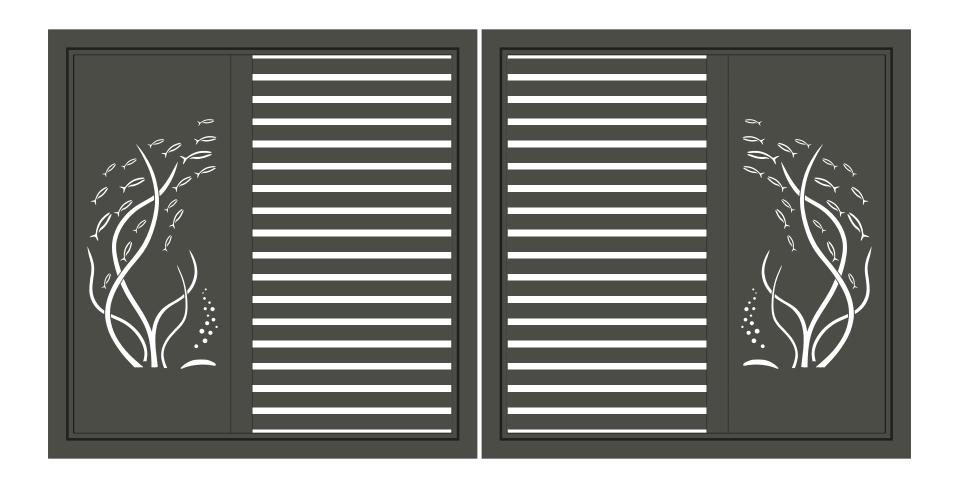
MAIN FRAME - Easy gate main frame 92x48x3. Mitred corners with welded 3mm thick corner braces giving 6mm wall thickness at each corner. INFILL - 65x16 horizontal slats at nominal 15mm spacing (adjust to suit your requirements). Decorative panel can be adjusted to anywhere in the gate. FINISH - Pre treatment and powder coat. Kit includes covers to conceal all infill fastening points. SIZE RESTRICTIONS - Sliding maximum width 6450mm. Swing maximum width 3200mm.
