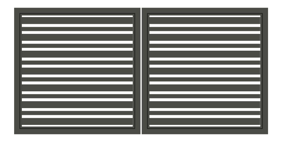
MAIN FRAME - Easy gate main frame 92x48x3. Mitred corners with welded 3mm thick corner braces giving 6mm wall thickness at each corner. INFILL - Alternate 65x16 and 38x16 horizontal slats at nominal 15mm spacing (adjust to suit your requirements).
