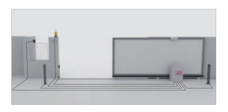
The above represented installation does not include safety devices such as safety edges. Their addition depends upon the risk assessment made on any installation in accordance with EN 12445-12453 standards.
